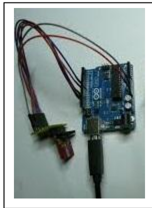
Figure 11: NRF device connected to Arduino
